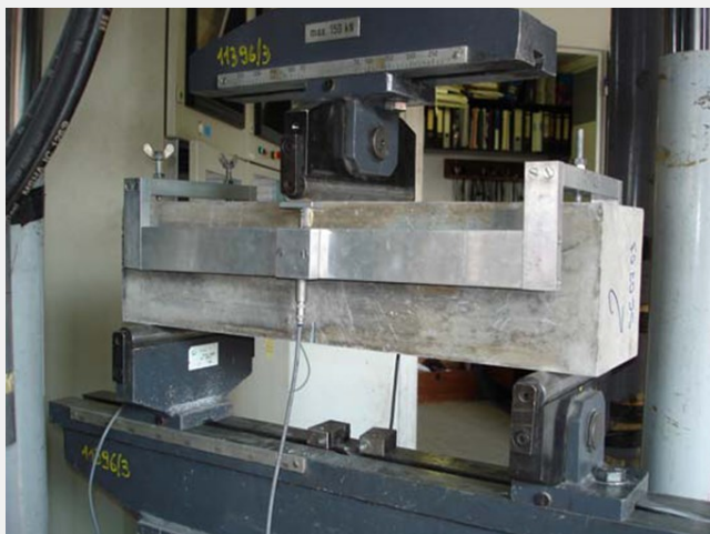
Beam test according to EN 14845-2
